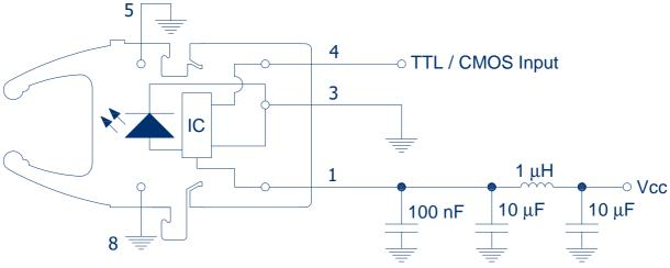
FIGURE 2 Recommended transmitter application circuit. See note 7 Table 6
