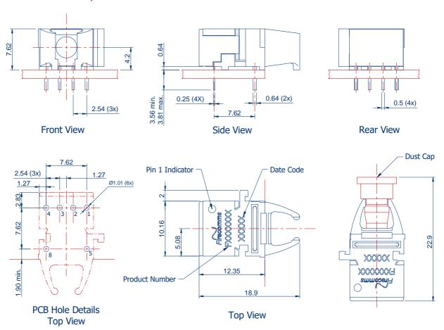
FIGURE 4 Mechanical dimensions of the horizontal connectors and PCB footprint, which is a top view General dimensional tolerance is  $\pm\,0.2~\text{mm}$
