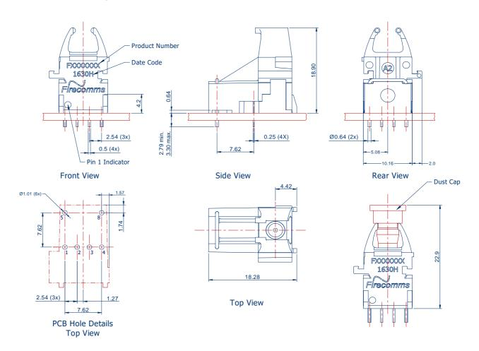
FIGURE 6 Mechanical dimensions of the vertical transmitter connectors and PCB footprint, which is a top view General dimensional tolerance is  $\pm\,0.2$  mm
